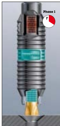
Phase 1: Small peak loads will be absorbed by the Torsion zone of the adaptor.
